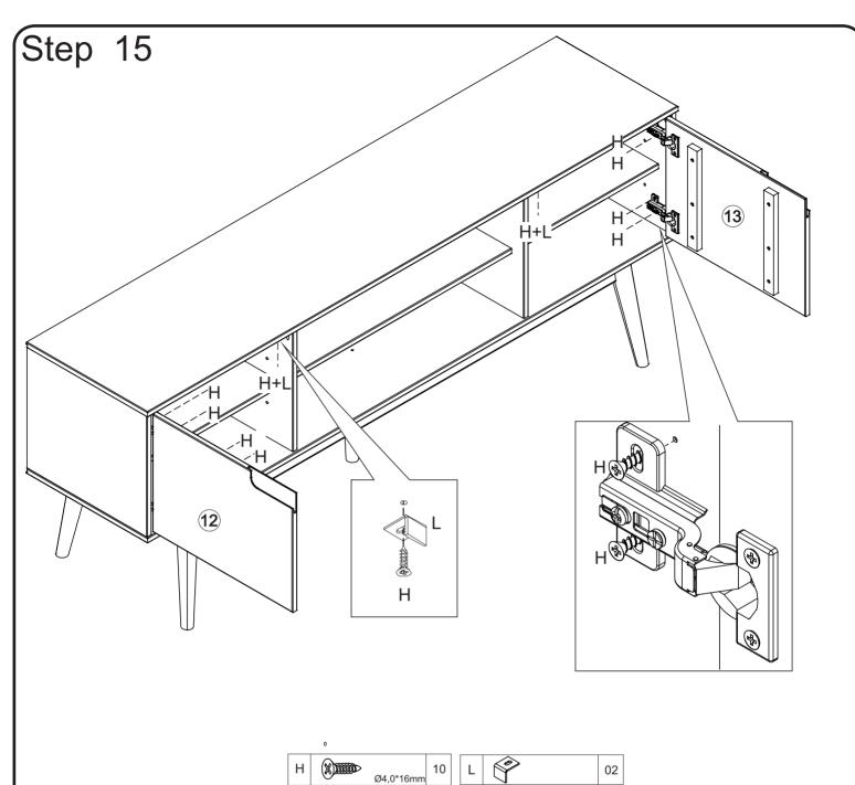
Secure part (12), (13) to part (2) and (3), with screw (H). Attach hardware (L) part (1), with screw (H).
